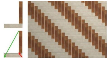
Illustration 15 Creating a "herringbone" tile layout"
