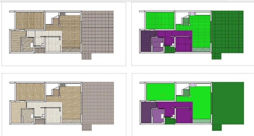
Illustration 60 Different representations of tiled areas - from left: texture with grout outline, color with grout outline, texture without outline, color without outline
