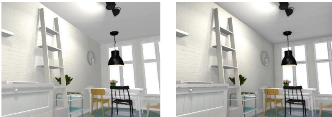
Illustration 3 Left: scene without global shading, right: with global shading (visible shadows at the junction of walls and ceiling)
