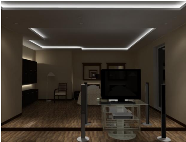
Fig. 293 – using Raytracing: raytracing of refracted rays is responsible for natural look of the glass TV stand, and the raytracing of reflected rays is in the multiply reflections in the mirror (10x)
