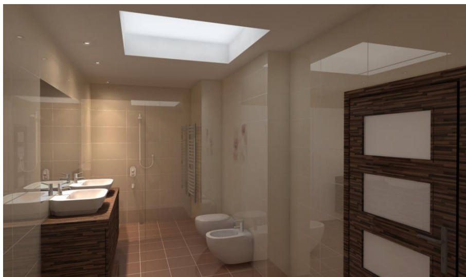
Fig. 307 - PROFESSIONAL RENDER: The same 3 halogen lights were used but the skylight has been attributed with the real light emission, what can be clearly seen on the edges of ceramic objects. Please notice the difference of a light distribution and colours in both cases.
