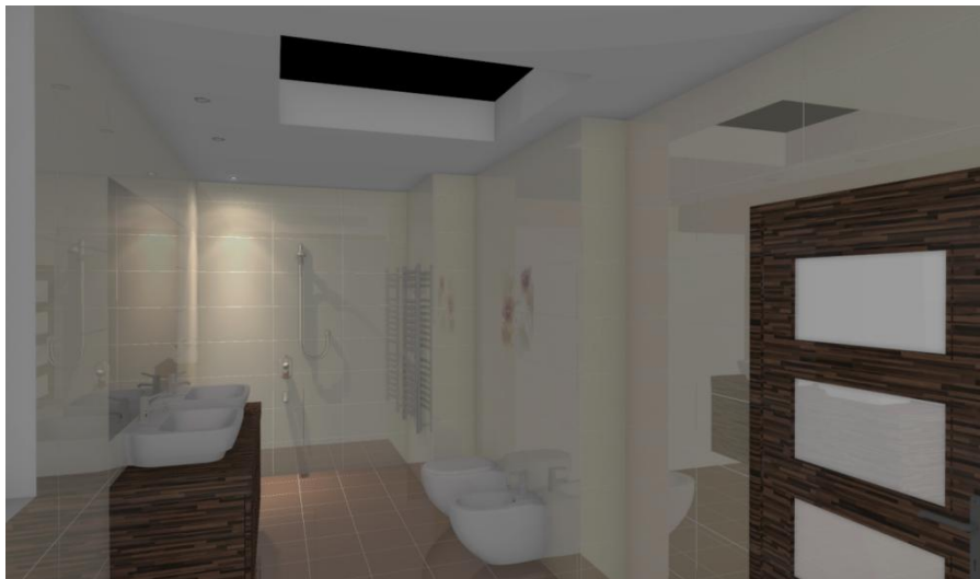
Fig. 304 - STANDARD RENDER: Only one halogen light has been used to light up this scene. It was necessary to use additional lighting up effect (the Brightness feature), because the scene was underexposed. In all cases exactly the same tiles were used – the differences in visible colours are caused only by the differences in light distribution.
