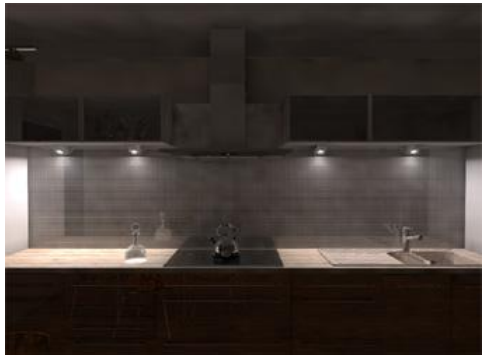
Fig. 260 – a scene with direct and indirect light – it is clearly seen that the light falling on the worktop reflects from it and illuminates the bottoms of the upper cabinets.
