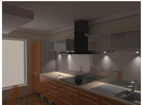
Fig. 266 – GI calculations for a scene with incorrectly drawn objects – it is clearly seen that the objects previously marked with a magenta colour are unnaturally dark
